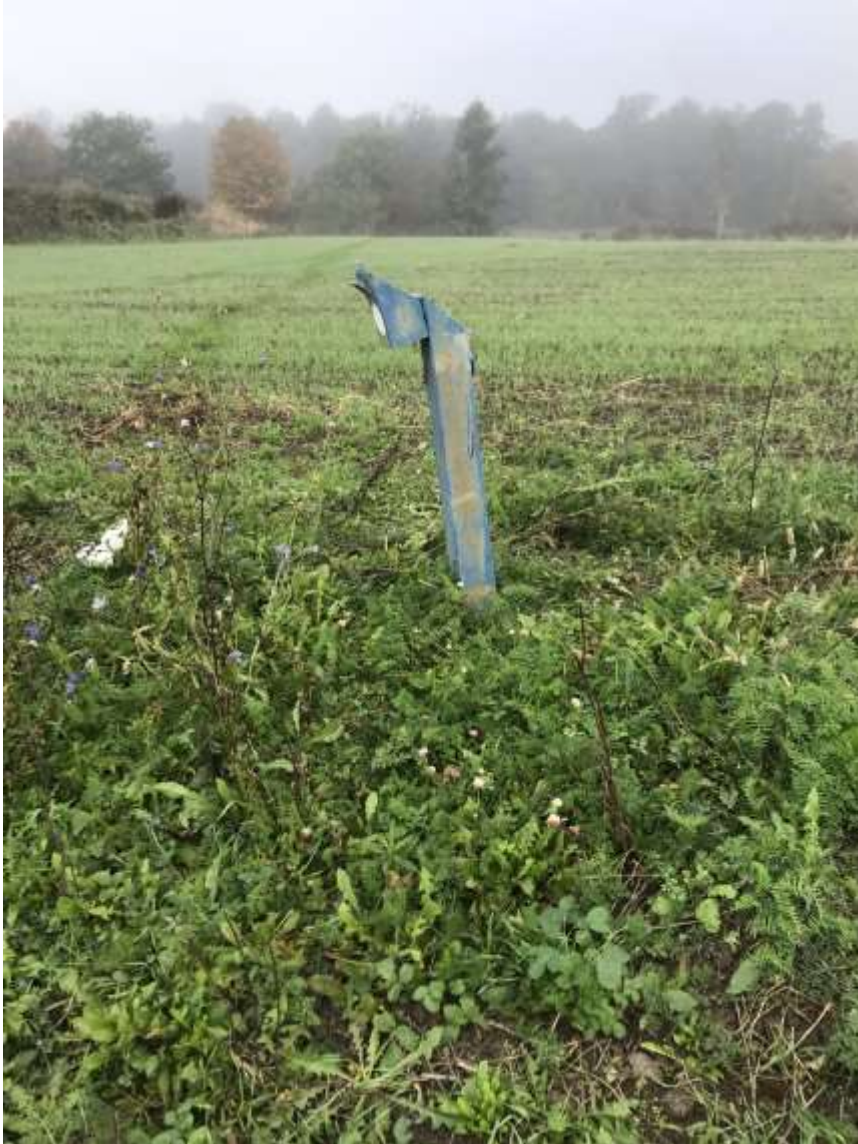
Photo 5: view of OW11R1, damaged by tractor.
