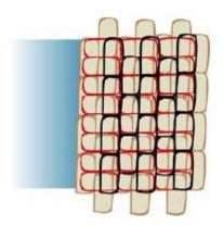
• Weave the polyethylene sheet between the courses of sandbags as to have at least two layers of sandbags protecting the polyethylene sheet from debris punctures. Maximum depth of the polyethylene sheet should be 3 sandbags or a quarter (1/4) of the cross section of the dike, whichever is less.
