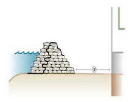
To create a more secure dike, when possible, create a trench in the soil that is one sandbag deep by two sandbags wide.
