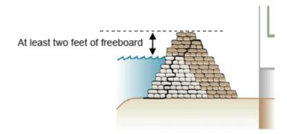
Sandbag dikes will compact when they get wet, which can reduce the available freeboard. The amount of compaction due to wetting increases with the size of the dike. Add at least five per cent to the required height of the dike to account for compaction. For example, add 3 - 4 inches for a six foot dike to account for compaction due to wetting.
