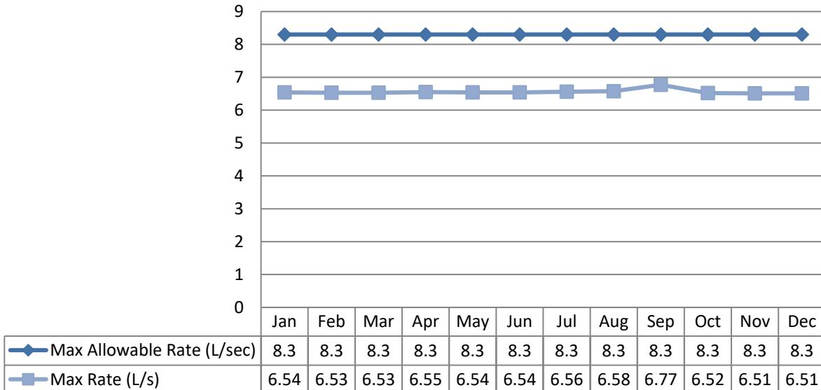
\* Flows increased instantaneously to 9.01 in October, 9.11 in November, and 9.30 in December but never exceeded 1 minute due to plant shutdown. The PTTW 500 L/Min was not exceed. The VFD issues caused these.
